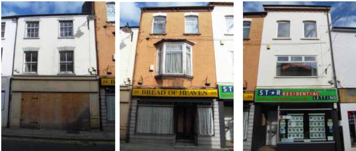
*These three adjacent buildings on Commercial Street display many of the concerns about poor building alterations and inappropriate replacement shop fronts. Loss of traditional window frames and window space; replacement roofing materials and loss of chimneys and pots; removal of heritage detail; and inappropriate/ unsightly replacement shop fronts and signage; with vacant floor space - demonstrate many of the problems seen throughout the Conservation Area.*
